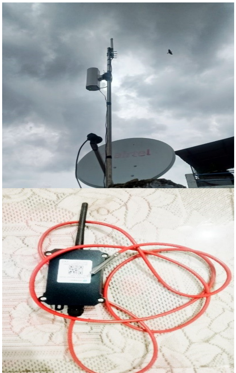
Fig. 3: LoRa Gateway and Sensor Node
